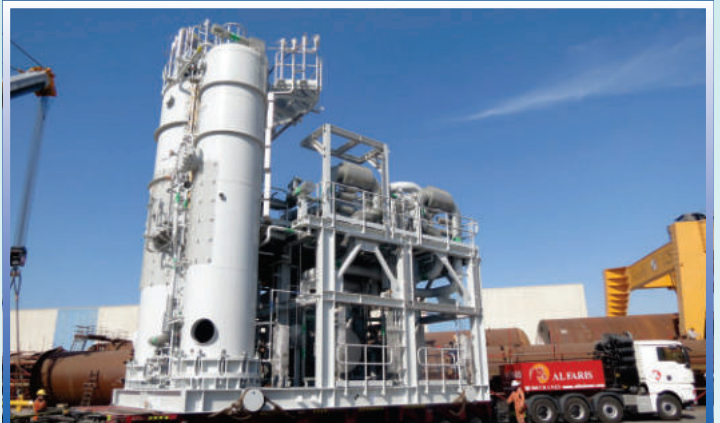
PRODUCED WATER & SAND TREATMENT PACKAGE
