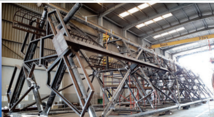
FLARE DERRICK STRUCTURE
